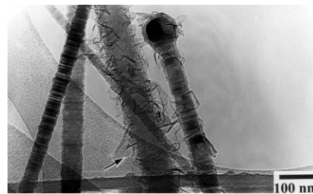
Fig. 5 Typical TEM image for the sample synthesized by nitrogen-transport HOPG–Ni catalytic growth. The arrow points to the disordered BN coated on \text{Si}_3\text{N}_4 nanowires.
